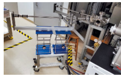
UHV Suitcase Transfers: Photo of the UHV suitcase during a device transfer from the glovebox to the low-temperature Raman system. The UHV suitcase is attached to the back of the glovebox.
