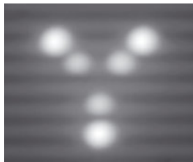
STM image of a dangling bond OR gate made of three pairs of atomic silicon dots.
