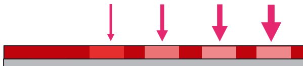
Figure 3: Grayscale exposure of thin film resist (FT ≤ 5 µm)
