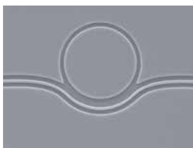
A channel waveguide coupled to a ring resonator. The waveguide is approximately 320 nm wide, the resonator diameter is 3 μm. The exposure laser wavelength was 405 nm. Design created with [1].
